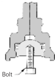
Remove disc insert by pulling on bolt
